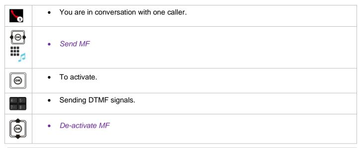
The function is automatically cancelled when you hang up. During a conversation, you can activate and deactivate the DTMF mode by pressing the \* key (long press).
