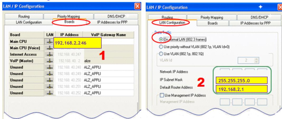
The ["Boards" Tab](#) shows the IP address for the main CPU and the default gateway. The main CPU IP address must be edited there ①
