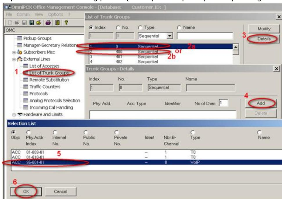
As a configuration variant, at step 2 you can include the SIP trunk access into the OXO's main Trunk Group (i.e. step 2a for index #1) or into one of the secondary Trunk Groups (e.g. step 2b for index #2).
