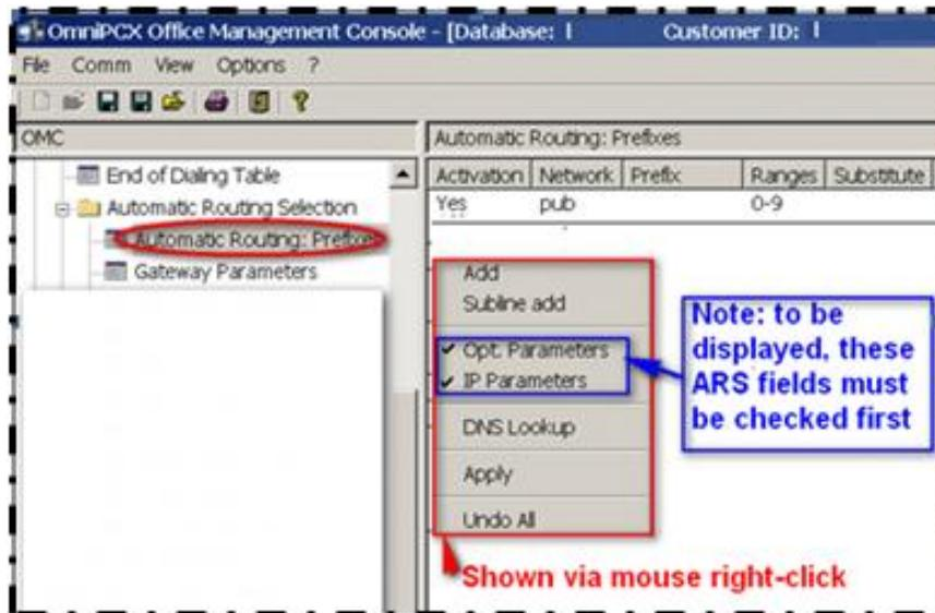
As illustrated in the following picture, first insert a route-line for standard calls (i.e. national/ international numbers): use the Add function to create a new line and then, configure the line parameters as indicated.
