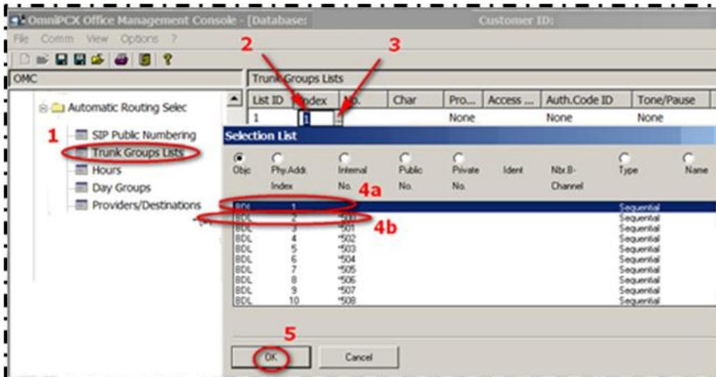
Carry out the selections and push-button steps 1 to 5 above. At step 4, you need to select the line index corresponding to a System Trunk Group previously defined at section 3.2.3 (i.e. selecting 4a for the Main Trunk Group or 4b for the secondary Trunk Group of index #2).
