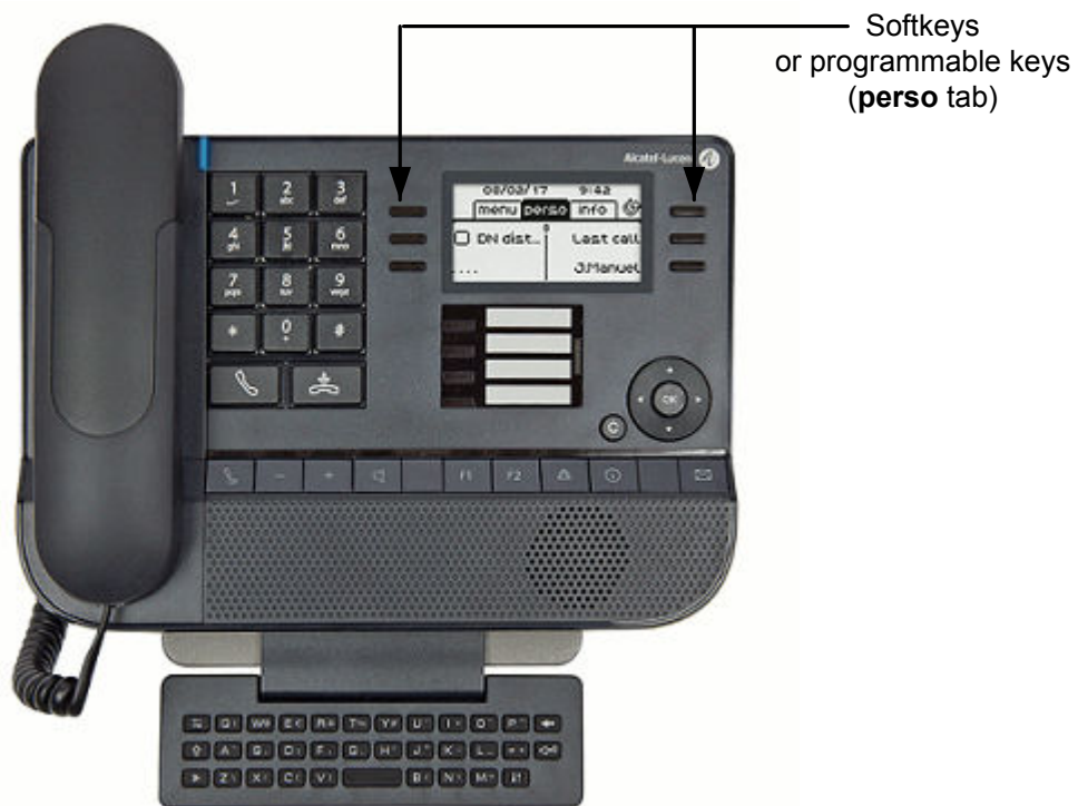
Figure 2.1: Key layout for 8028s Premium DeskPhone sets
